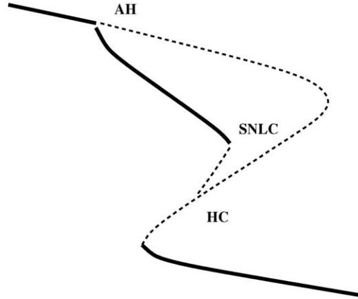
Fig. 10. An example of the bifurcation diagram for the fast subsystem (compare with Fig. 3). The stable limit cycles terminate through a SNLC bifurcation.
