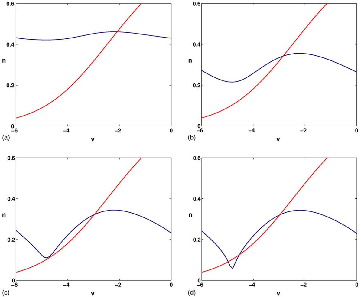
Fig. 2. The changes in the nullcline configuration for increasing values of  $\beta$  reflect the sequence of the bifurcations in the fast subsystem. A supercritical AH bifurcation takes place as the nullcline configuration in (a) changes to that in (b). Plots in (c) and (d) correspond to a SN and a HC bifurcations respectively.
