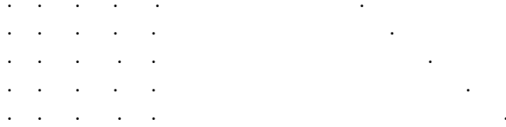
FIG. 1.1. Data arrays structures: Full MIMO square transfer function (data from all sources at all receivers) (left) vs monostatic data (data received only back at each source, typical of SARs) (right).
